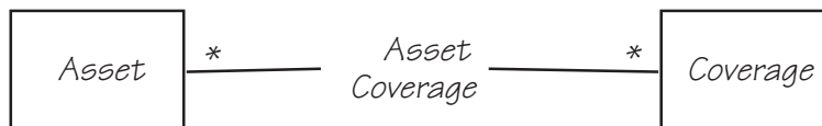
Figure 10: This generic model covers all valid business combinations of Asset Types and related Coverage Types. Every Asset can have an Asset Coverage connection with many types of Coverage. And every type of Coverage could be connected via an Asset Coverage relationship to many types of Assets.
